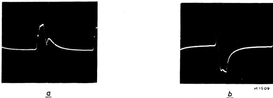
Fig.34. Oscillograms of the sum voltages of the synchronisation pulses and the flyback pulses at the anode (a) and at the cathode (b) of the phase splitter tube.
