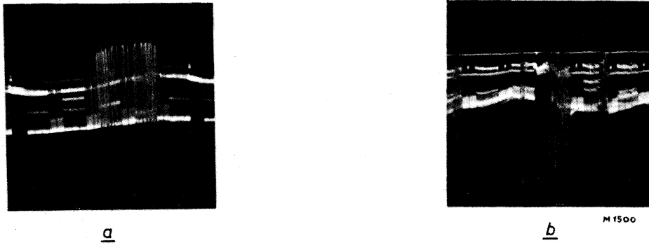
Fig.28. (a) Video signal with positive-going interference pulses. (b) After the output signal of the noise inverter has been added to a video signal, the polarity of the interference pulses is reversed.
